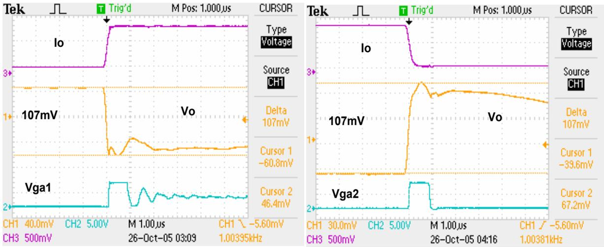
Fig.3.5.7 Improved transient waveforms @ 5~80A, 550A/ $\mu$ s
