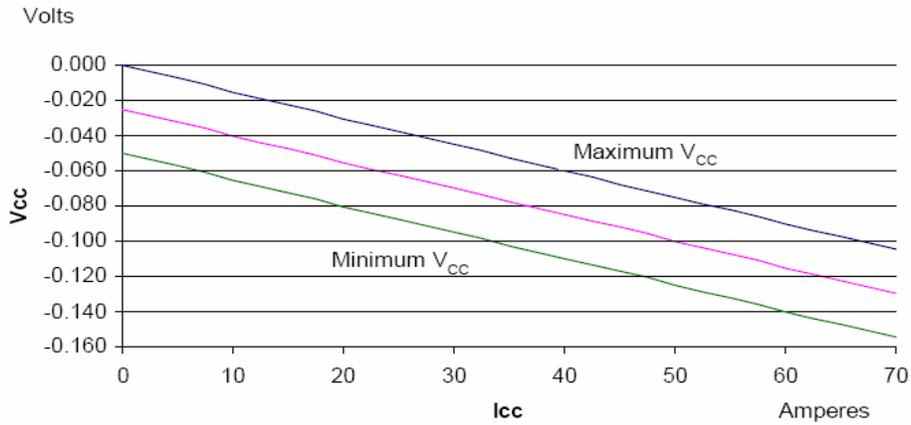
Fig.1.2.5 Intel Pentium 4 processor socket load line
