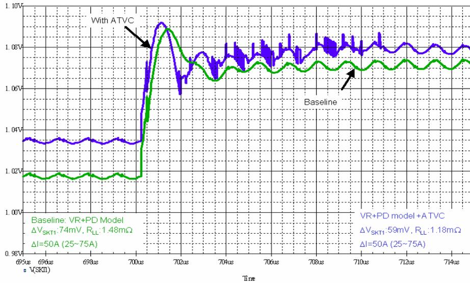
Fig.3.3.10 Parallel ATVC simulation results in step-down load
