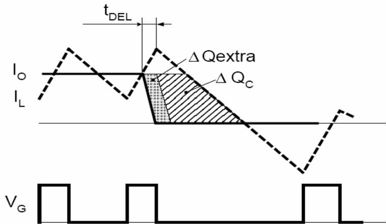
Fig.1.2.4 Delay time  $t_{DEL}$  impact on voltage spikes
