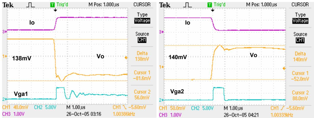
Fig.3.5.9 Improved transient waveforms @ 5~100A, 550A/ $\mu$ s
