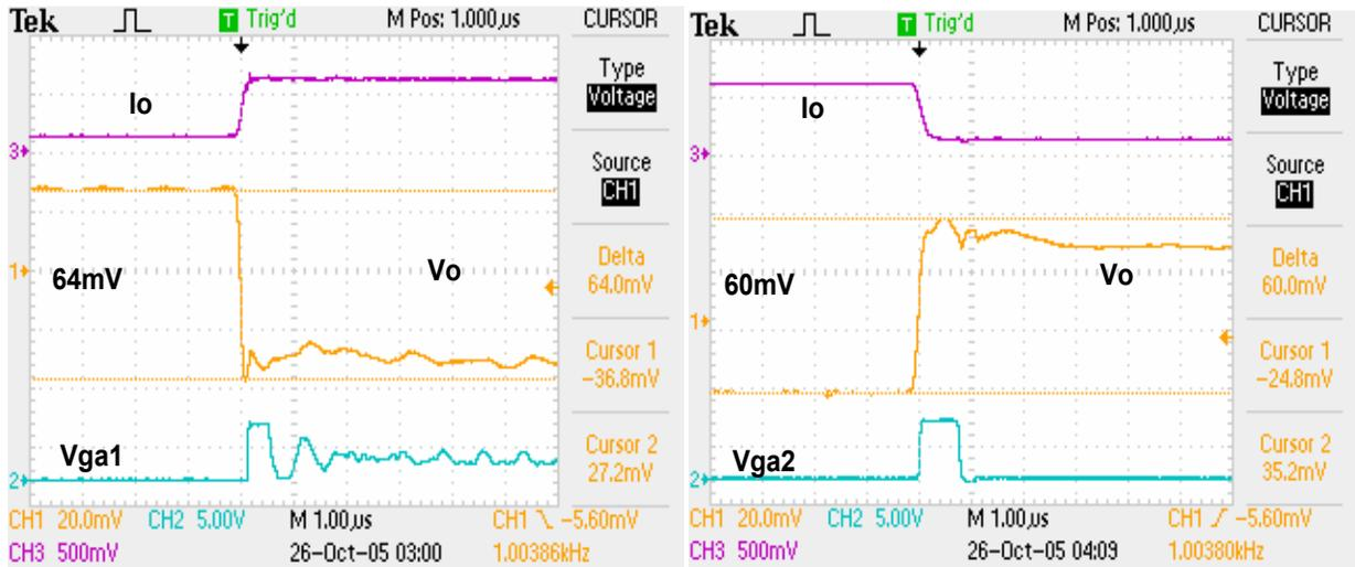
Fig.3.5.5 Improved transient waveforms @ 5~50A, 550A/ $\mu$ s
