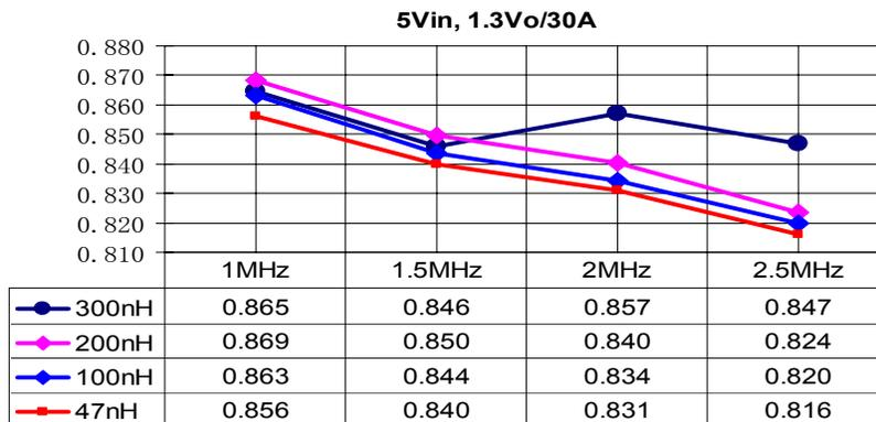
Fig.3.1.8 Tested efficiency @ 5Vin, 1.3Vo/30A
