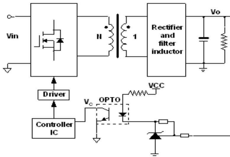
Fig. 4.1.1 Isolated DC-DC converter with primary side control
