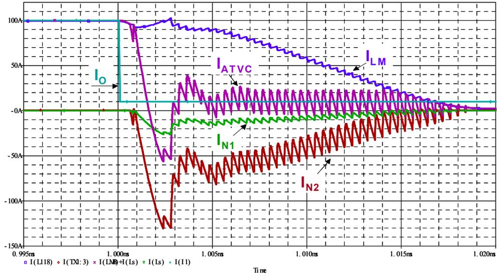
Fig.3.3.6 Parallel AVTC current waveforms in step-down load
