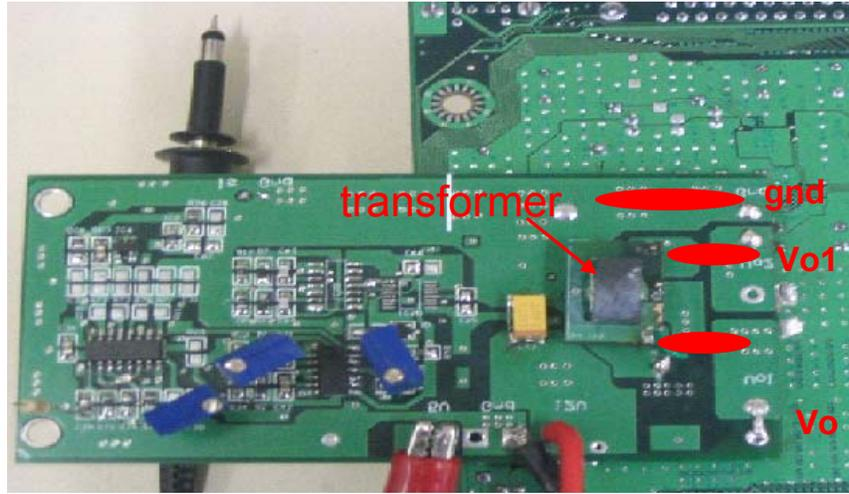
Fig.3.3.3 ATVC prototype on Intel motherboard
