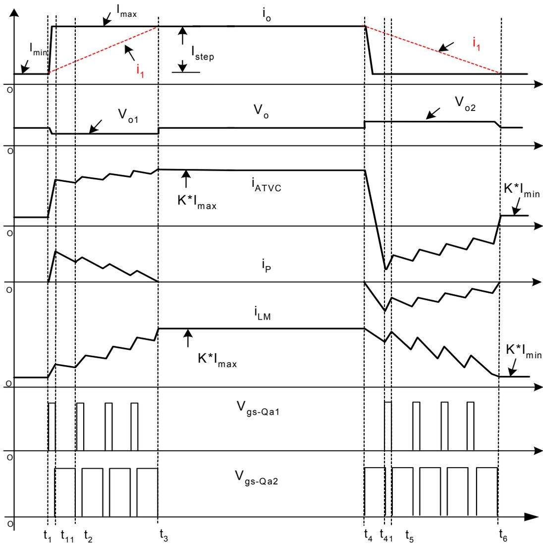
Fig.3.1.5 Operation waveforms of Parallel ATVC
