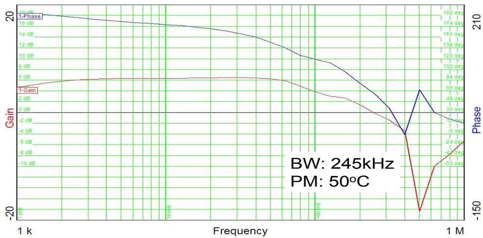
Fig.3.5.13 Tested ATVC bode-plot in CCM
