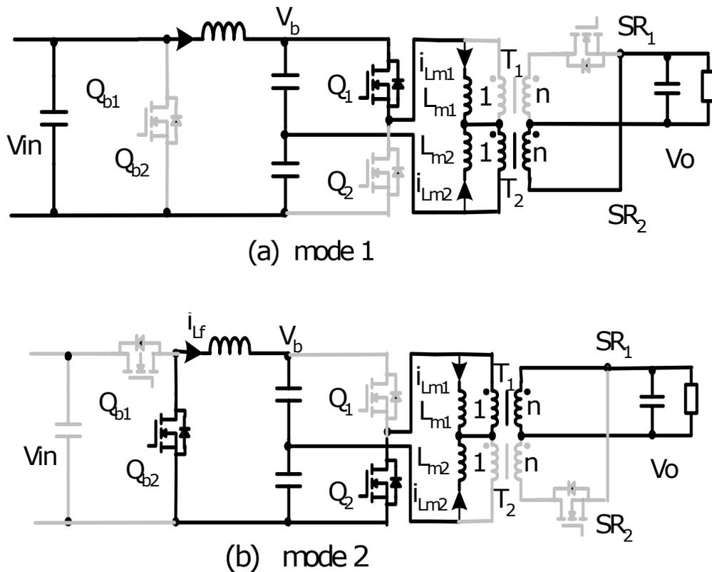
Fig.4.2.8 Operations analysis of experimental prototype
