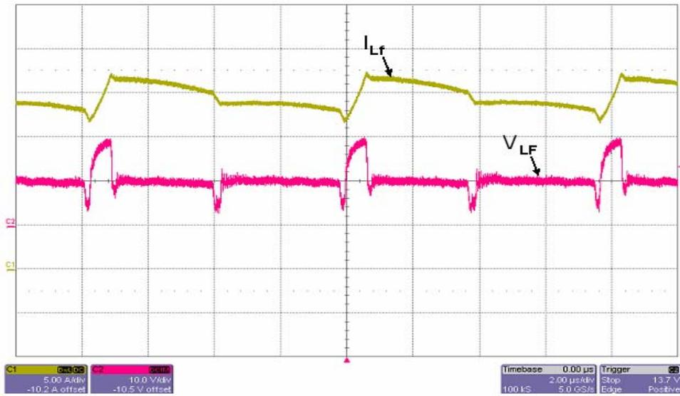
Fig.4.4.15 Waveforms of rectified voltage and filter current
