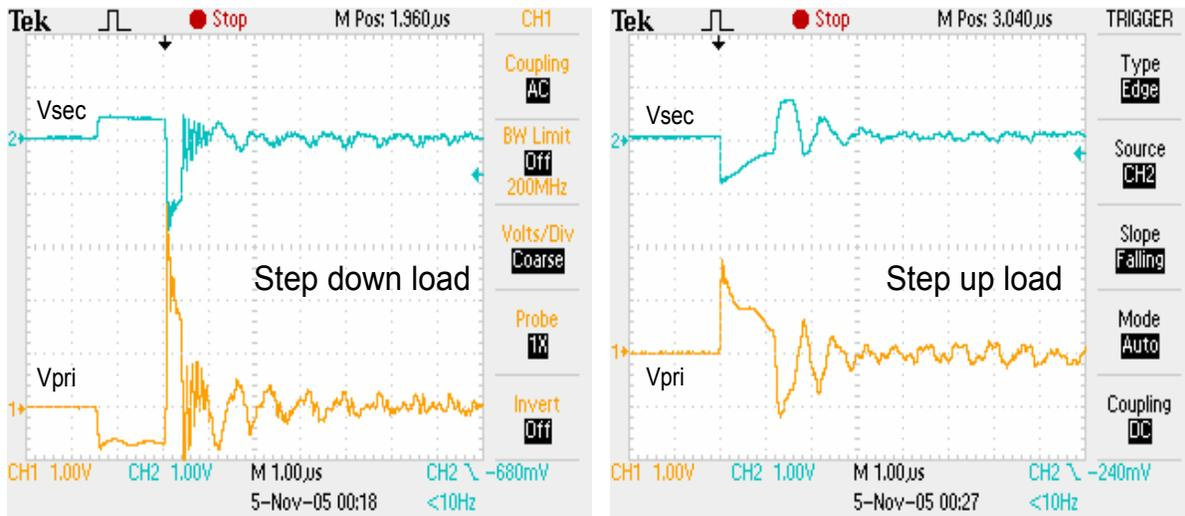
Fig.3.5.12 Average injected transient voltage waveforms
