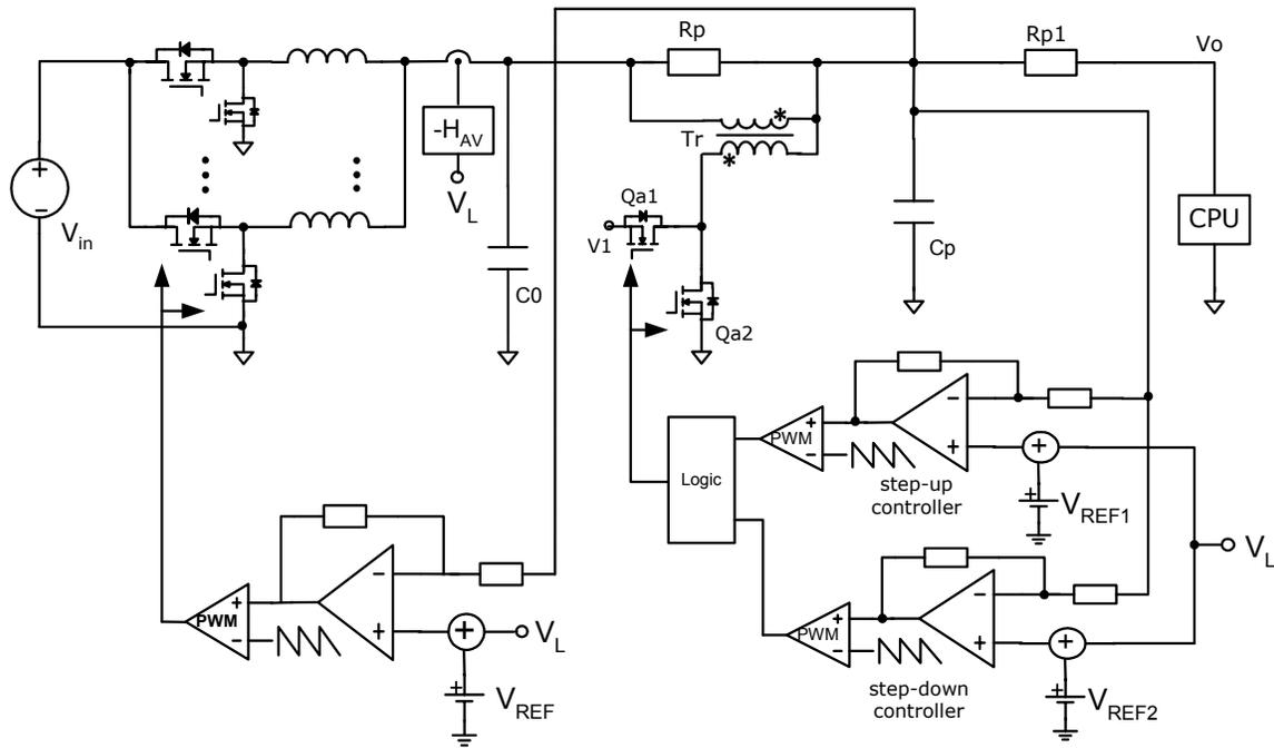
Fig.3.2.1 VR and parallel ATVC controller block diagrams
