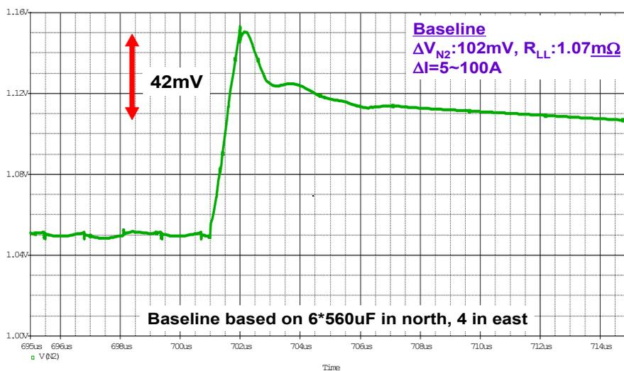
Fig.3.3.12 LGA775 baseline load line in step-down load
