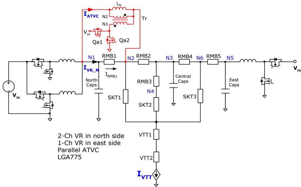
Fig.3.2.6 CPU power distribution mode of LGA775 with parallel ATVC
