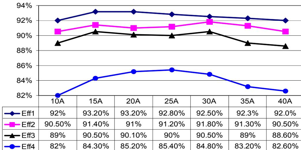
Fig.4.4.17 Tested efficiency of PPR and HB converter
