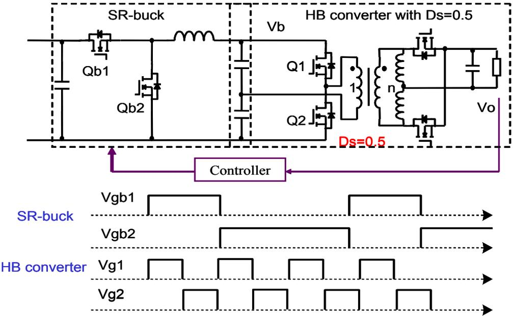
Fig.4.2.1 Synchronous buck and 0.5 duty cycle HB converter
