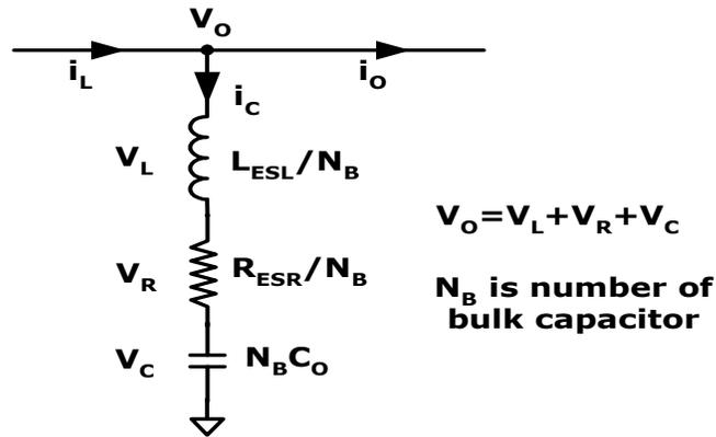
Fig.1.2.1 Simplified circuit for output voltage spikes estimation
