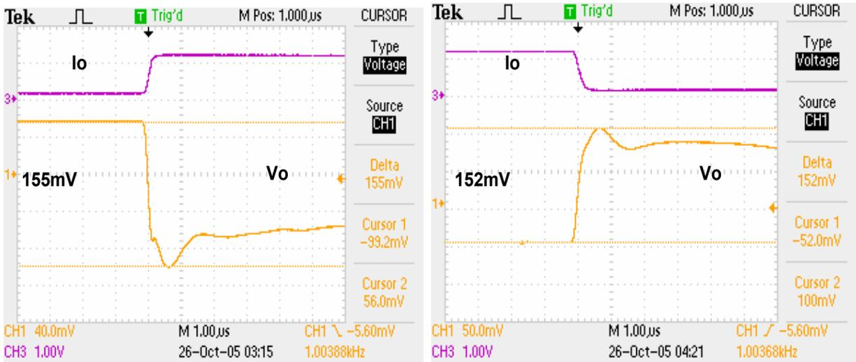
Fig.3.5.8 Baseline transient waveforms @ 5~100A, 550A/ $\mu$ s
