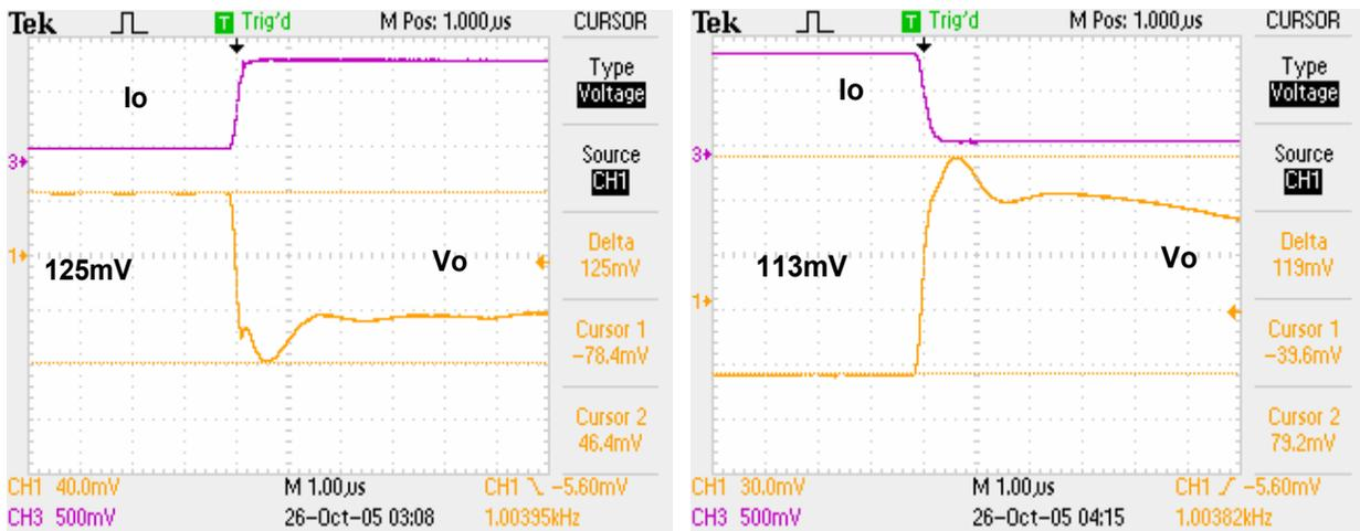
Fig.3.5.6 Baseline transient waveforms @ 5~80A, 550A/ $\mu$ s
