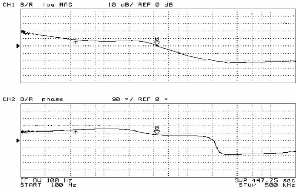
Fig.4.3.9 Experimental Bode Plot with balancing winding network
