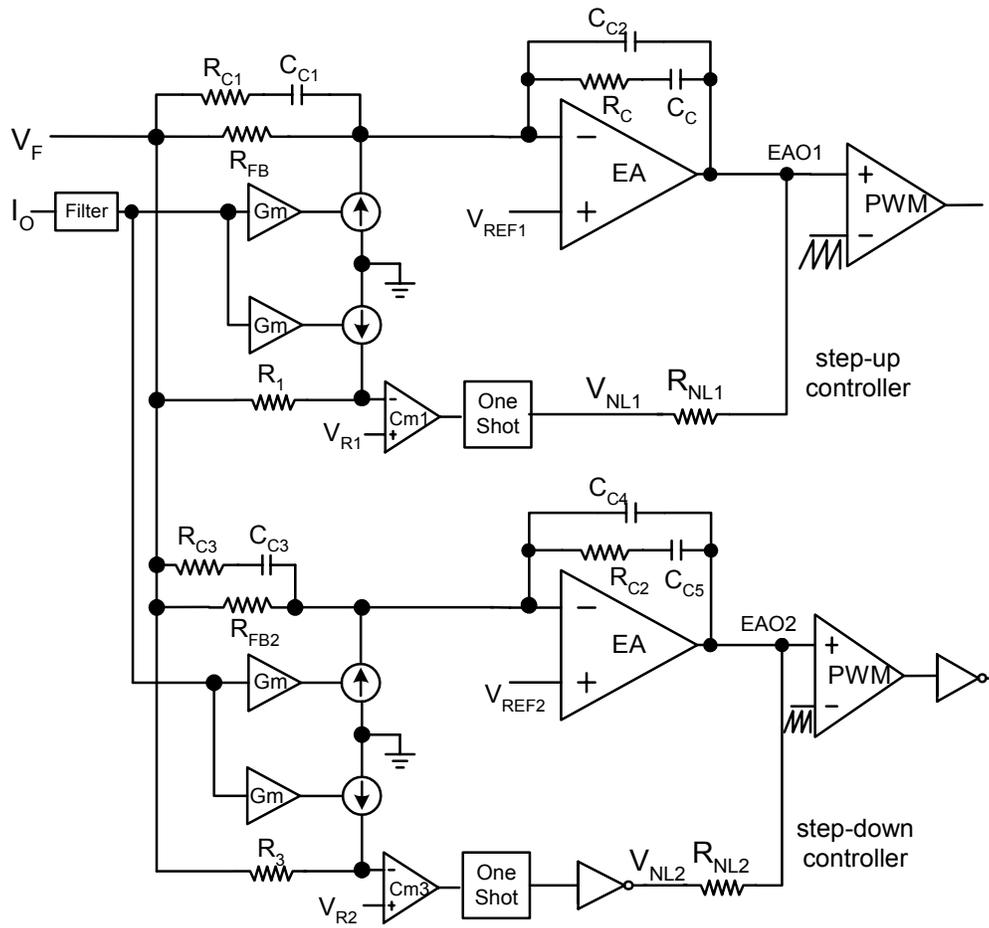
Fig.3.4.17 Control circuit block diagram for the ATVC
