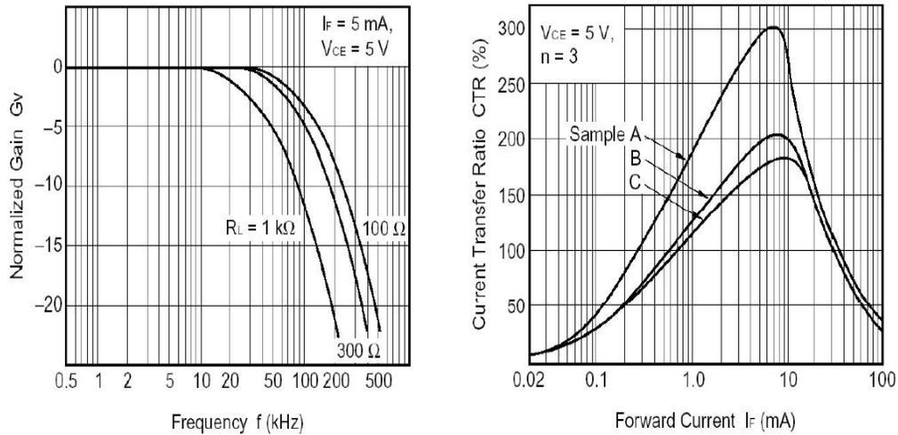
Fig.4.1.2 Optocoupler performance characteristics
