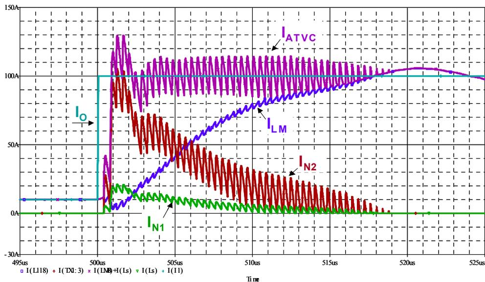
Fig.3.3.5 Parallel AVTC current waveforms in step-up load
