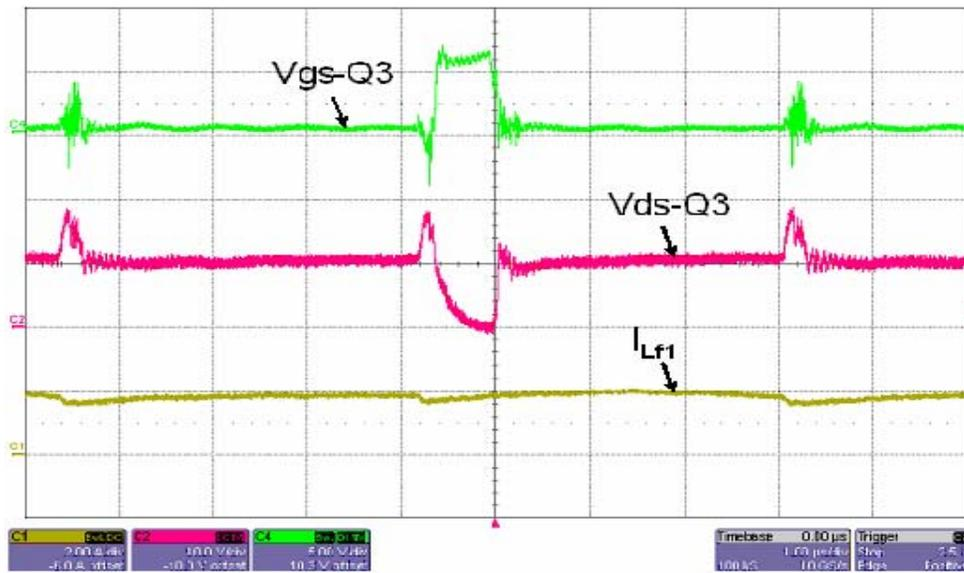
Fig.4.4.14 Voltage waveforms of  $Q_3$  and current  $I_{Lf1}$
