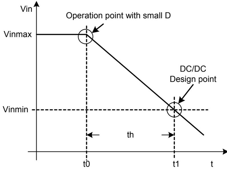
Fig.4.4.1 Wide range input DC-DC converter design
