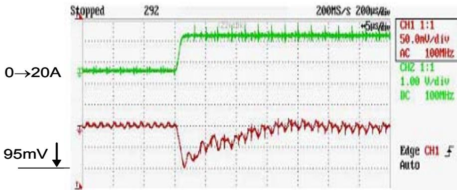
Fig.4.2.10 Output ripple in step-up load @10A/ $\mu$ s
