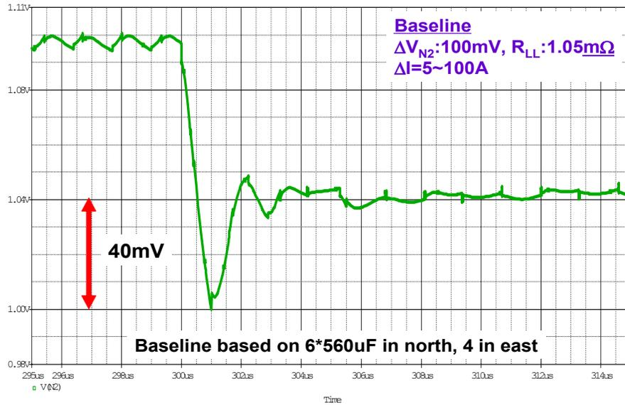
Fig.3.3.11 LGA775 baseline load line in step-up load
