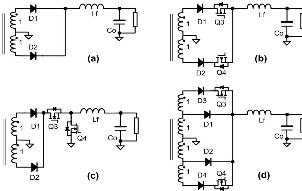
Fig.4.4.2 Different types of secondary side post regulator
