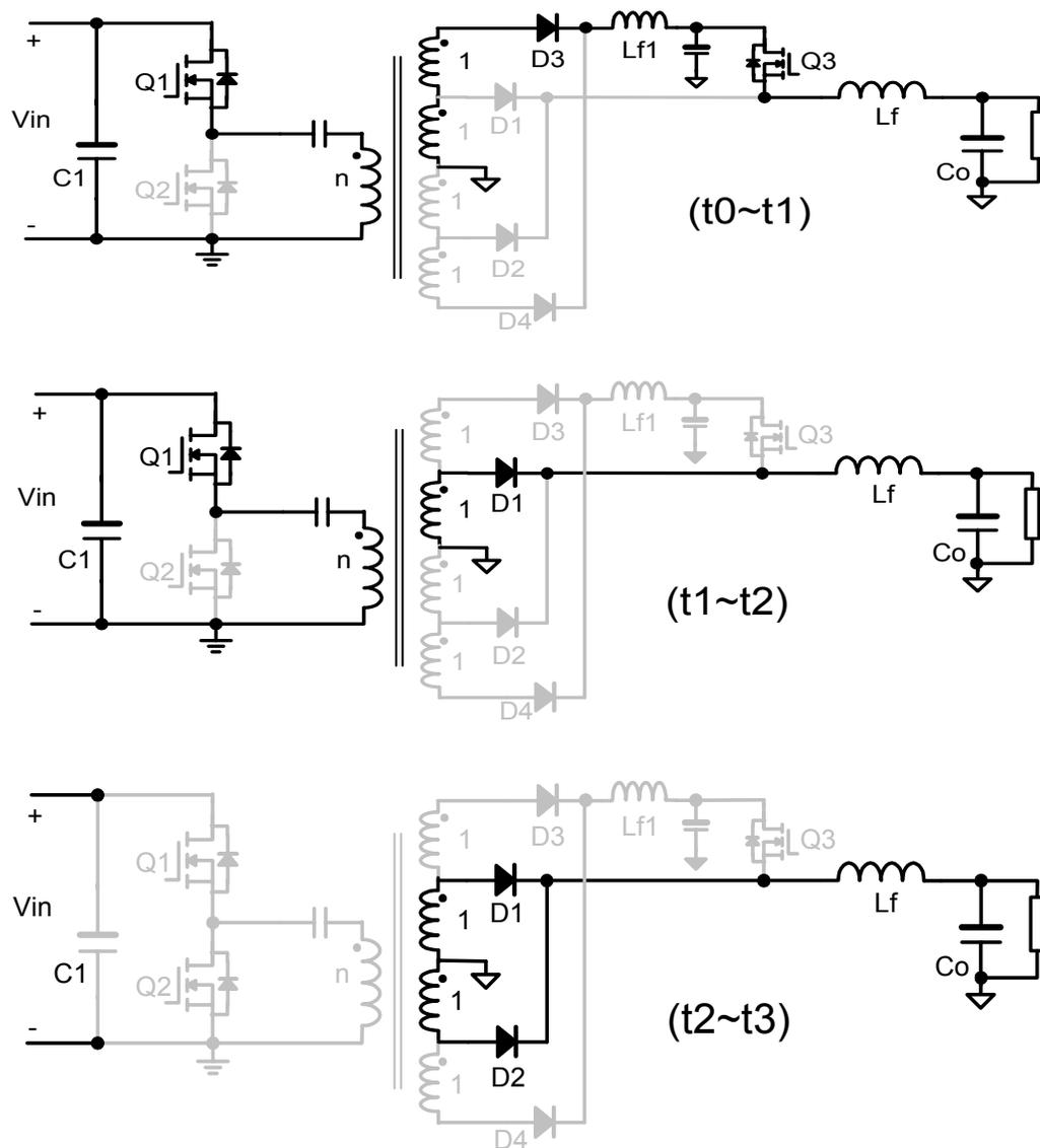
Fig.4.4.6 Detailed PPR operation analysis
