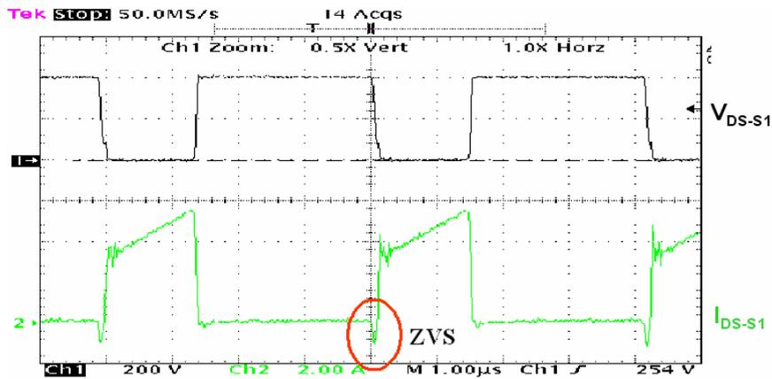
Fig.4.3.2 S1 ZVS in HBCC converter
