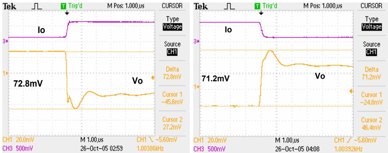
Fig.3.5.4 Baseline transient waveforms @ 5~50A, 550A/ $\mu$ s
