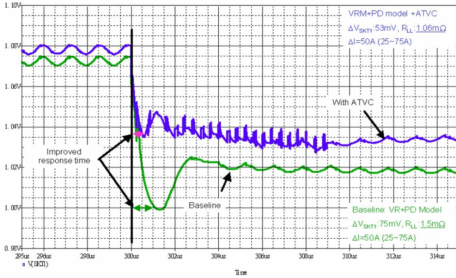
Fig.3.3.9 Parallel ATVC simulation results in step-up load
