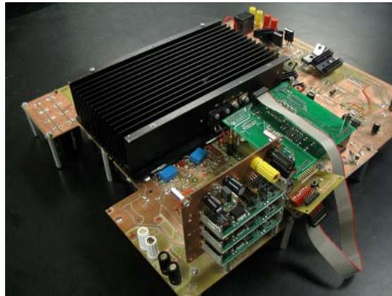
Figure 8.8: Prototype of 1kW Single-Stage High-Frequency Link Inverter System
