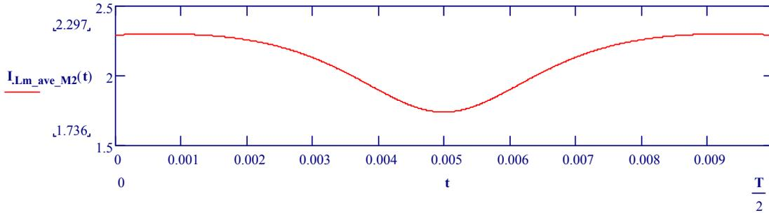
Figure 6-8 Average Flyback Magnetizing Current during Line Cycle
