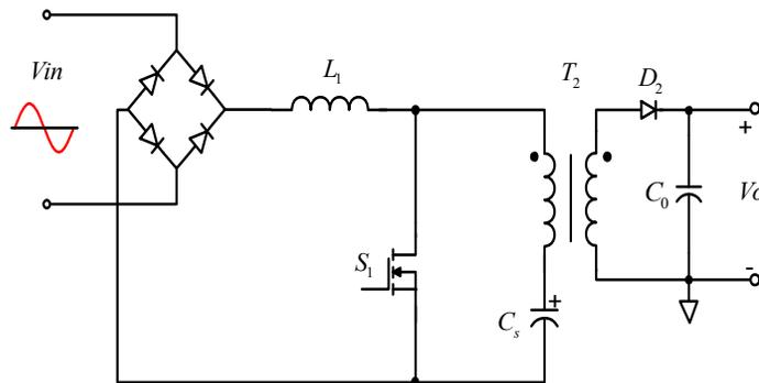
Figure 4-1 BIFRED Topology for Single-stage PFC Applications
