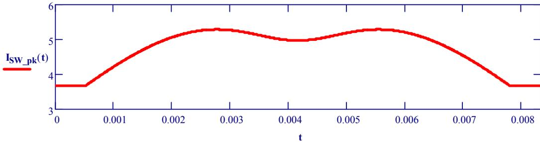
Figure 6-18 Maximum Switch Current during a Line Cycle
