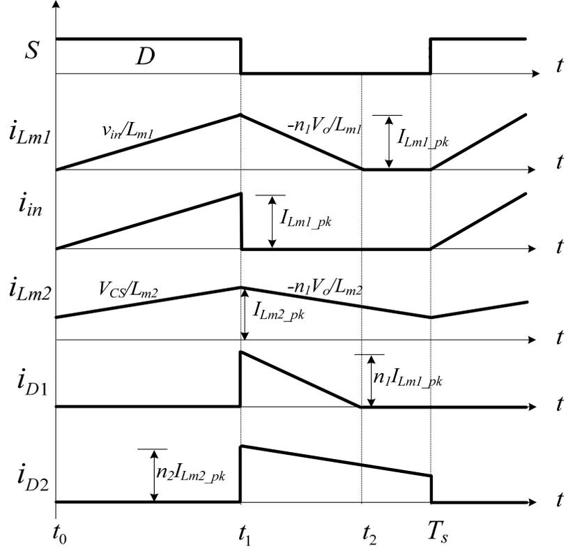
Figure 4-5 Key Waveforms during Flyback Mode Operation
