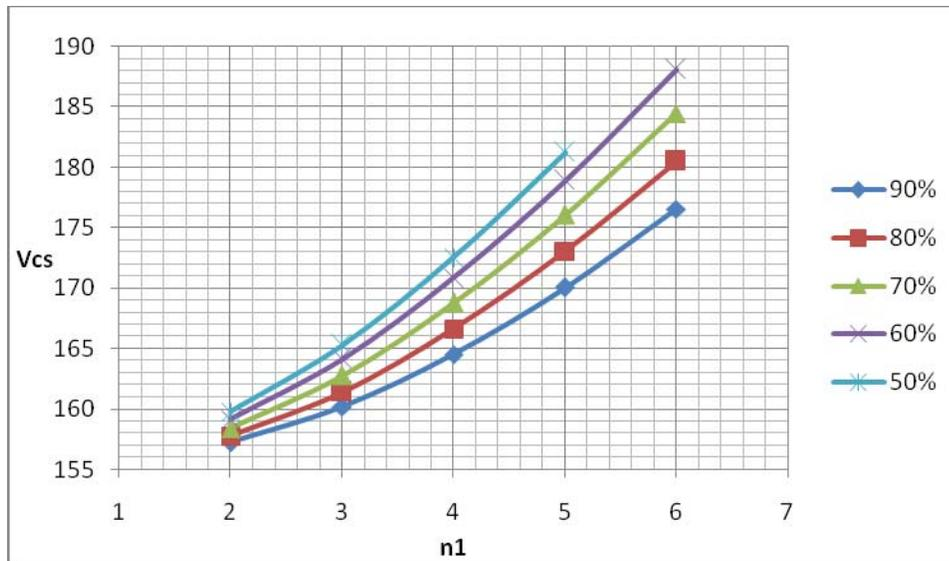
Figure 4-11 Bus Capacitor Voltage versus  $n_1$  for Different  $P_D$  Values
