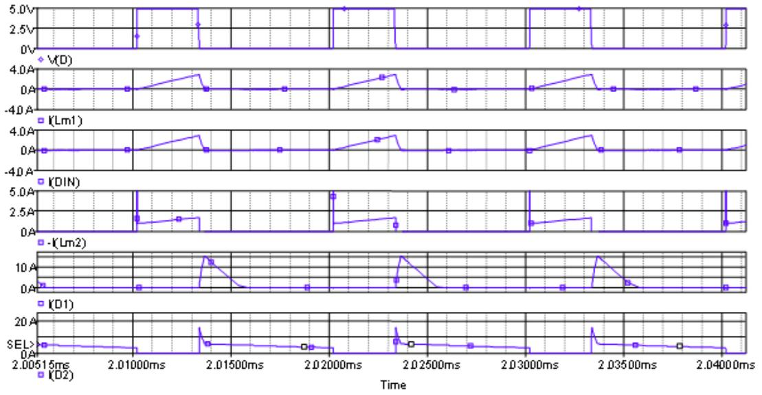
Figure 4-20 Simulation Waveforms during the Flyback Mode
