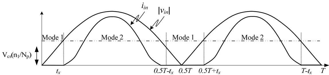
Figure 6-2 Modes of Operation during a Line Cycle
