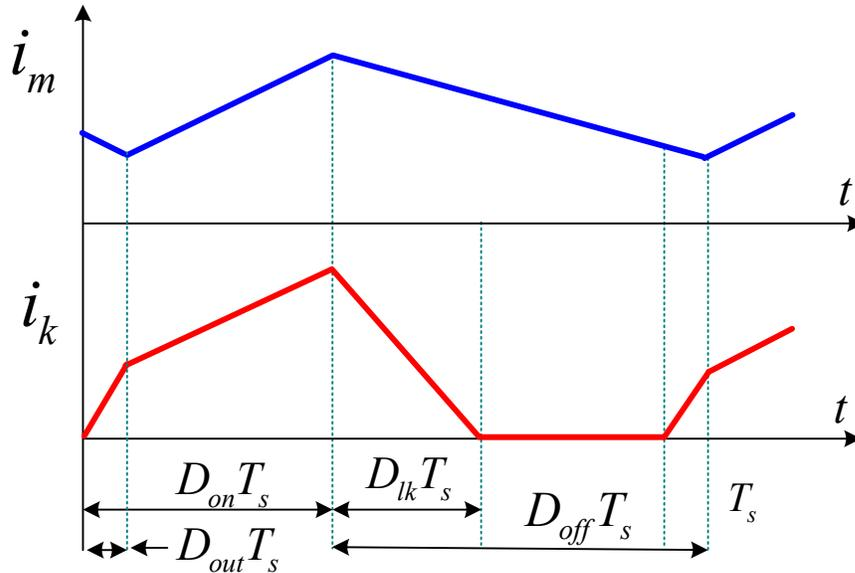
Figure 5-5 Time Duration Definition of the Proposed Model
