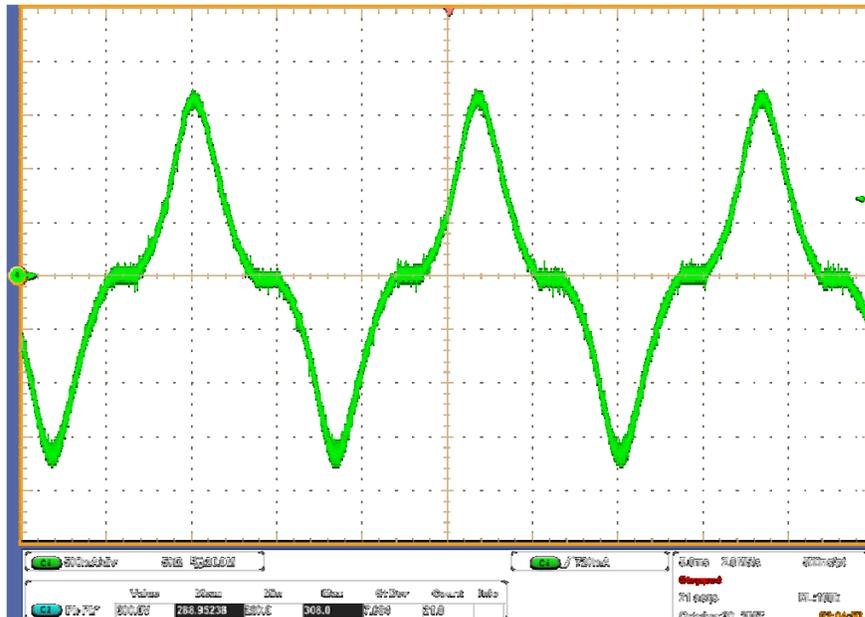
Figure 6-32 Input Current Waveform at 110Vrms under Full Load
