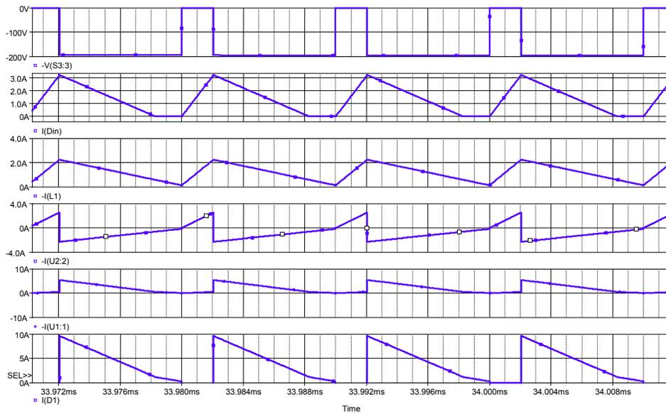
Figure 6-24 Simulation Waveforms during Mode 2 Operation
