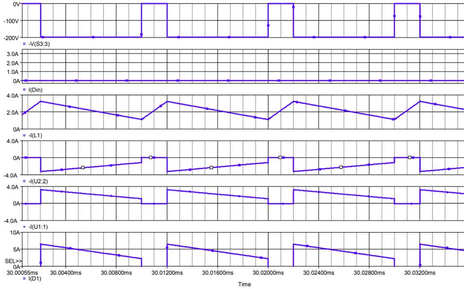
Figure 6-23 Simulation Waveforms during Mode 1 Operation
