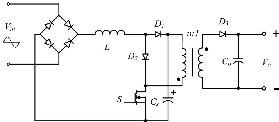
Figure 2-3 Single-stage Boost/Flyback Combination Circuit
