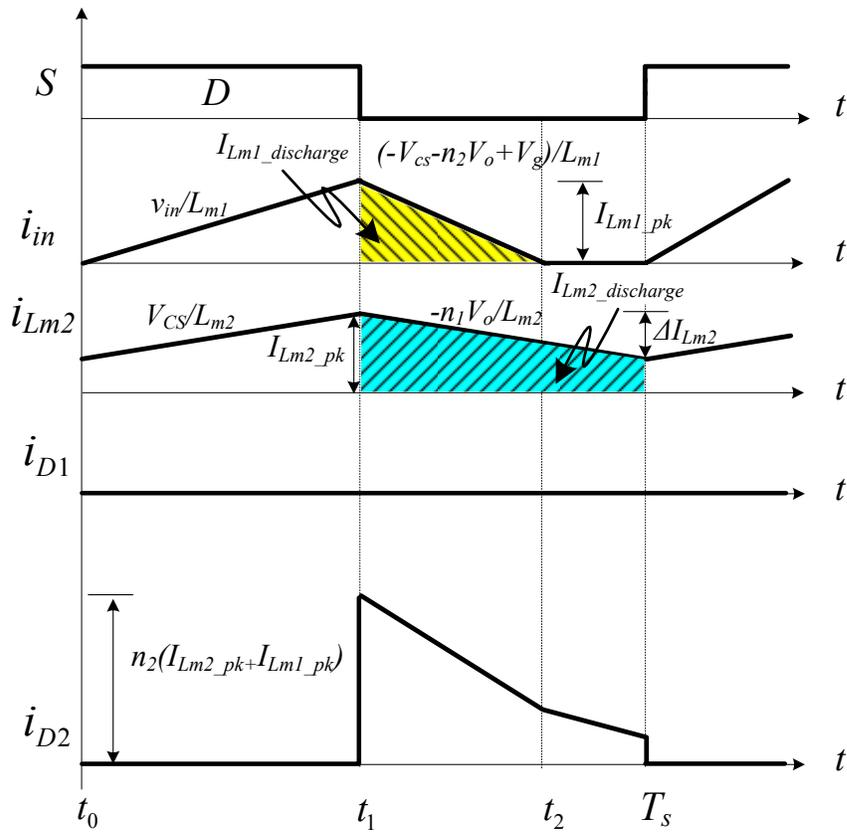
Figure 4-7 Key Waveforms during Boost Mode Operation
