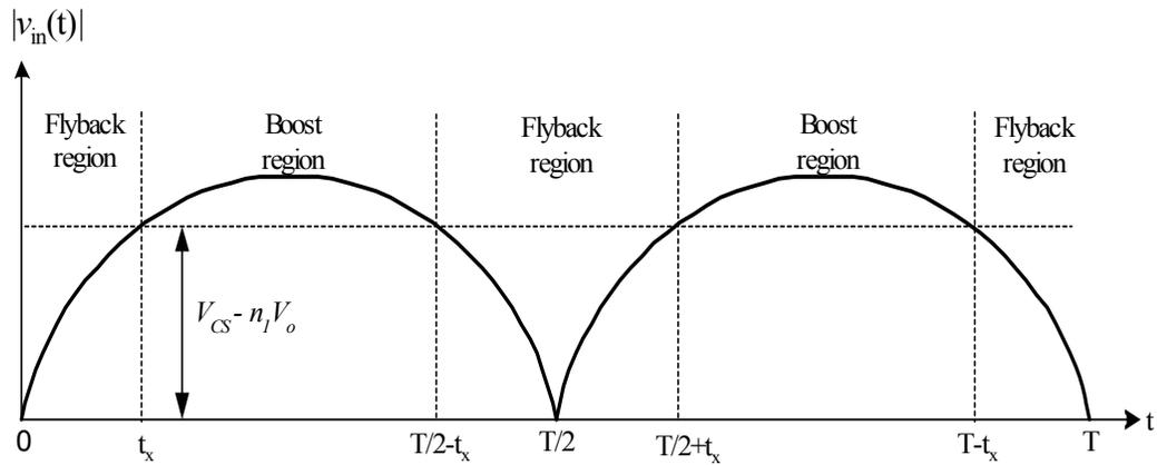
Figure 3-8 Regions of Operation During one Line Cycle
