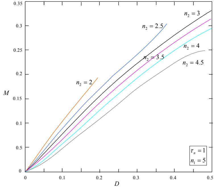
Figure 3-14 M vs. D under different  $n_2$  values
