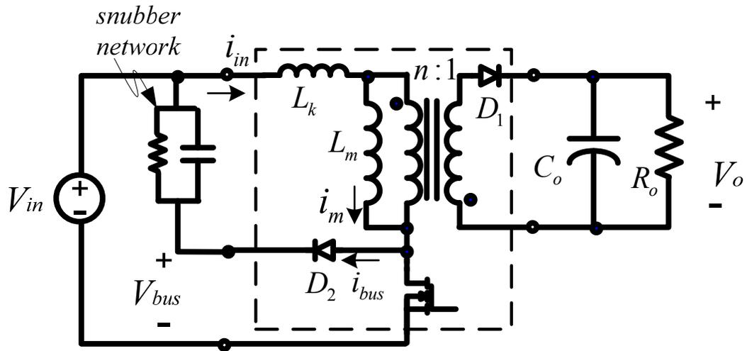
Figure 5-3 The Proposed Five-terminal Switched Transformer Model
