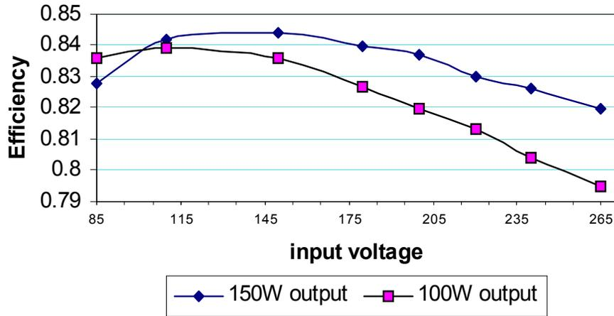
Figure 3-20 Efficiency versus Line voltage
