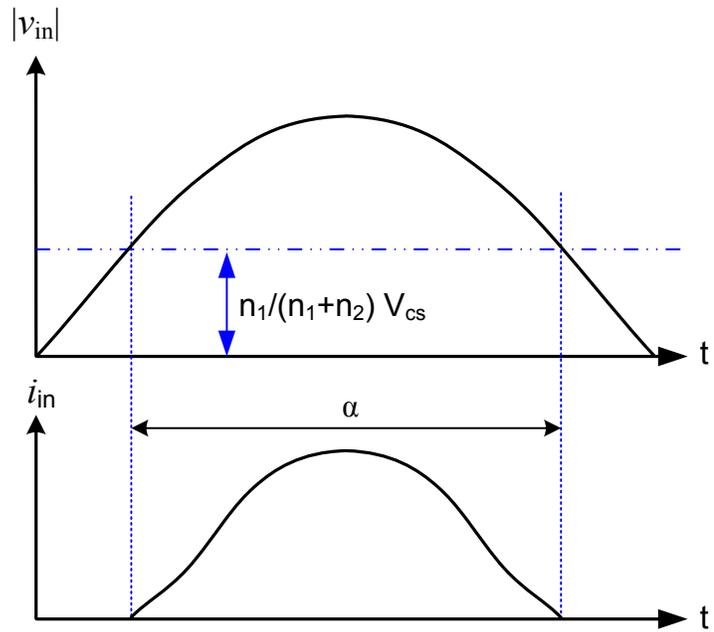
Figure 2-13 Boundary Modes of Operation during Half-line Cycle
