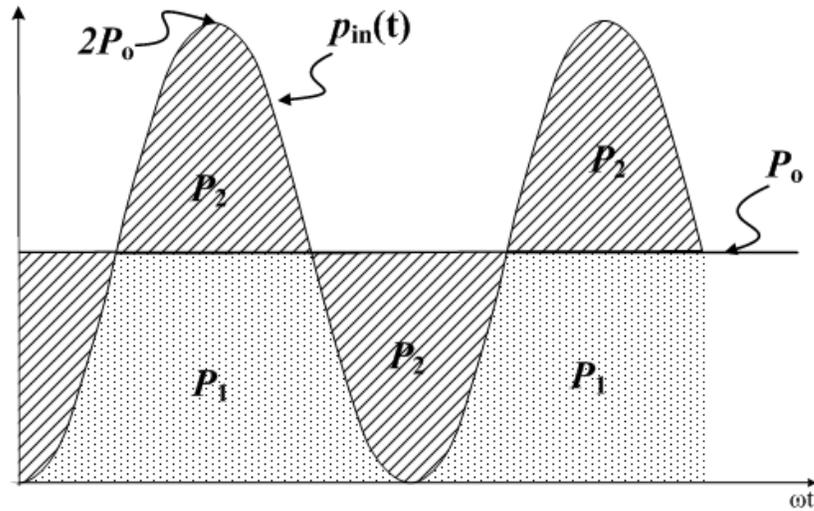
Figure 2-9 Power Relationship in Single-Phase PFC Converters
