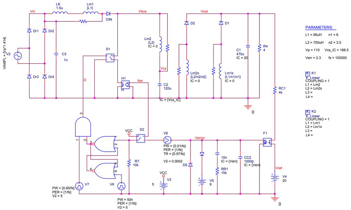
Figure 4-19 Simulation Schematics for the Bi-flyback Converter
