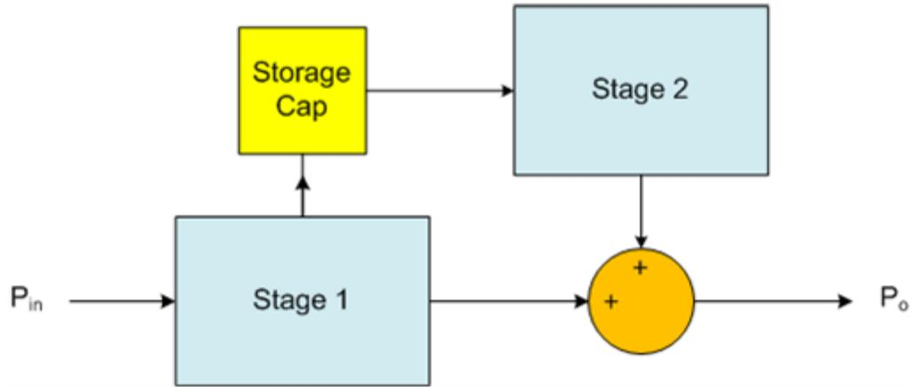
Figure 2-10 Block Diagram for the Direct PFC Scheme
