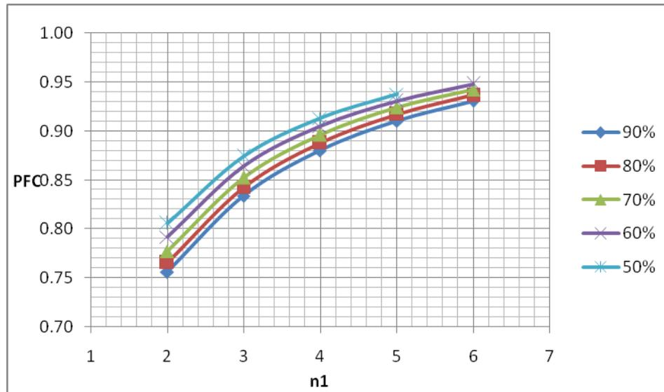
Figure 4-15 PF versus  $n_1$  for Different  $P_D$  Values
