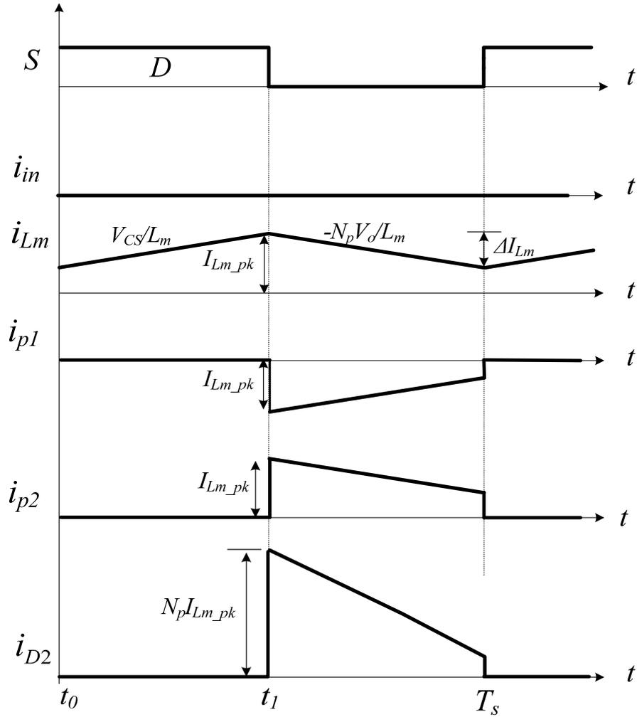
Figure 6-4 Key Waveforms during Mode 1 Operation
