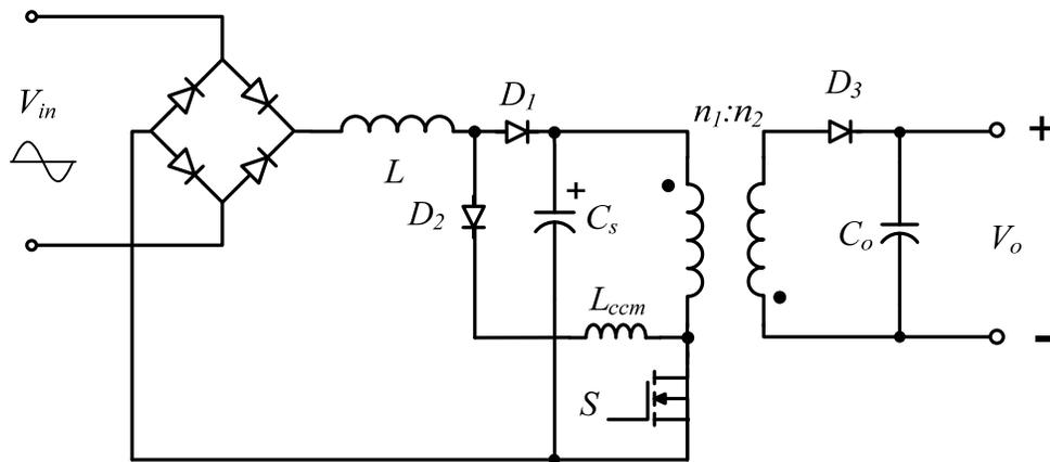
Figure 2-6 Current Source CCM PFC Circuit
