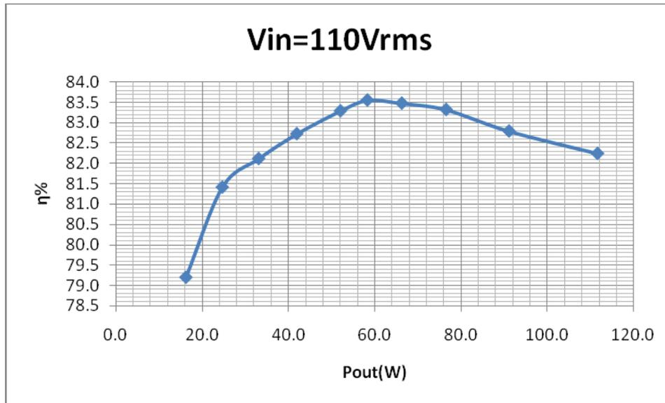
Figure 4-23 Measured Efficiency versus Output Power at 110Vrms
