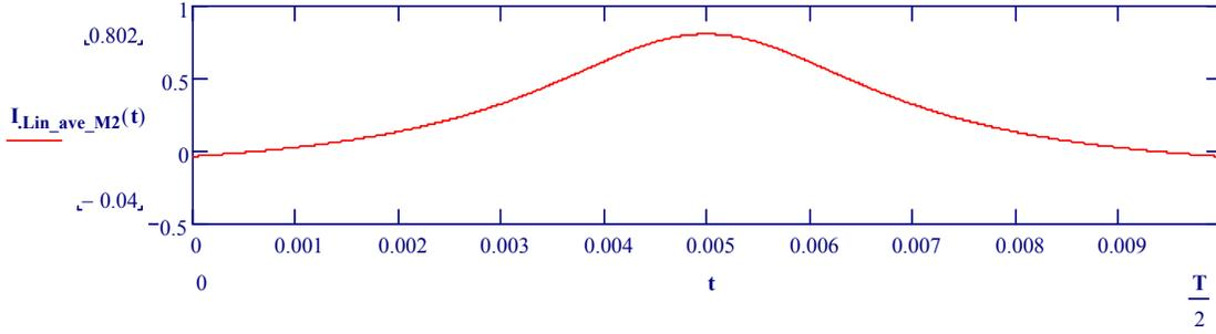
Figure 6-7 Average Input Current during Line Cycle
