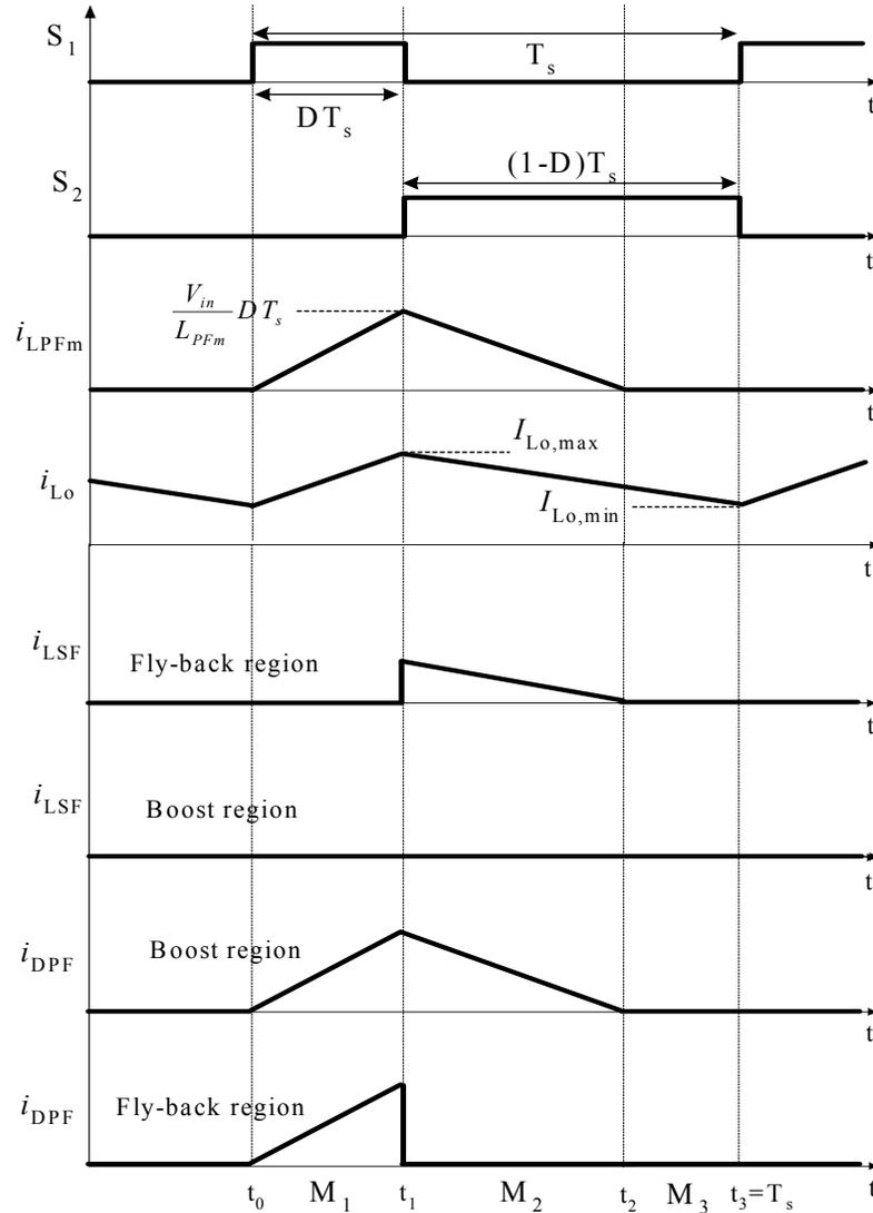
Figure 3-10 Operation Waveforms
