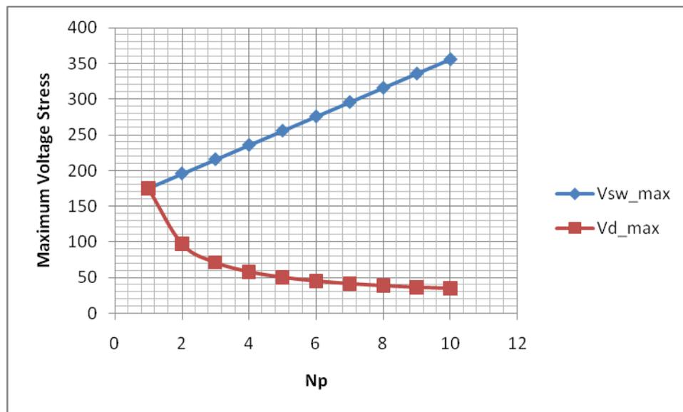
Figure 6-19 MOSFET and Diode Voltage Stress versus  $N_p$
