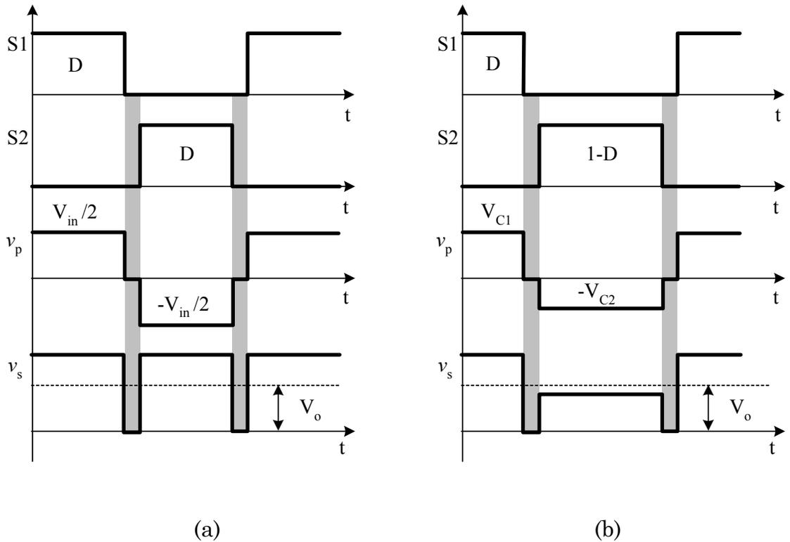
Figure 3-2 Switching Waveforms: (a) Symmetric witching, (b) Asymmetric switching
