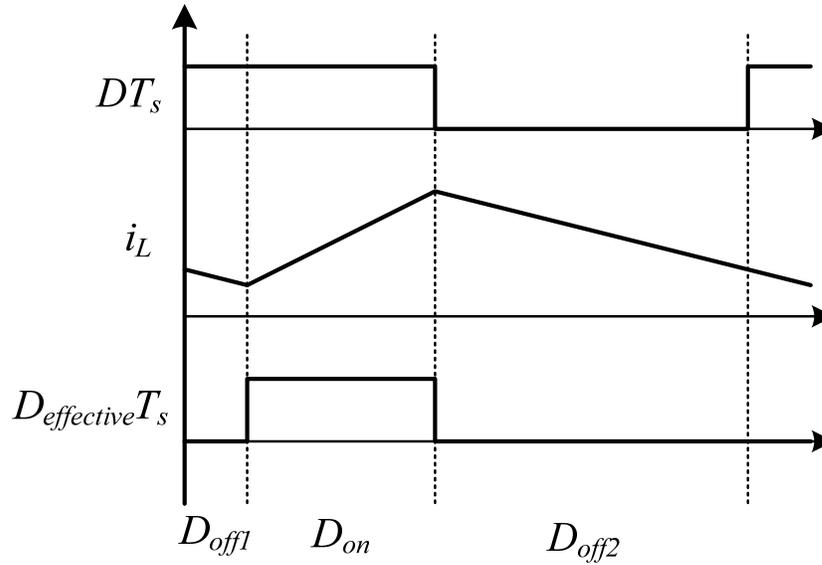
Figure 2-7 Effective Duty Cycle in Single-Stage PFC
