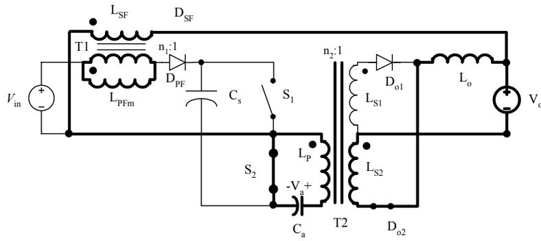
(b) Flyback Mode 2:  $t_1 < t < t_2$
