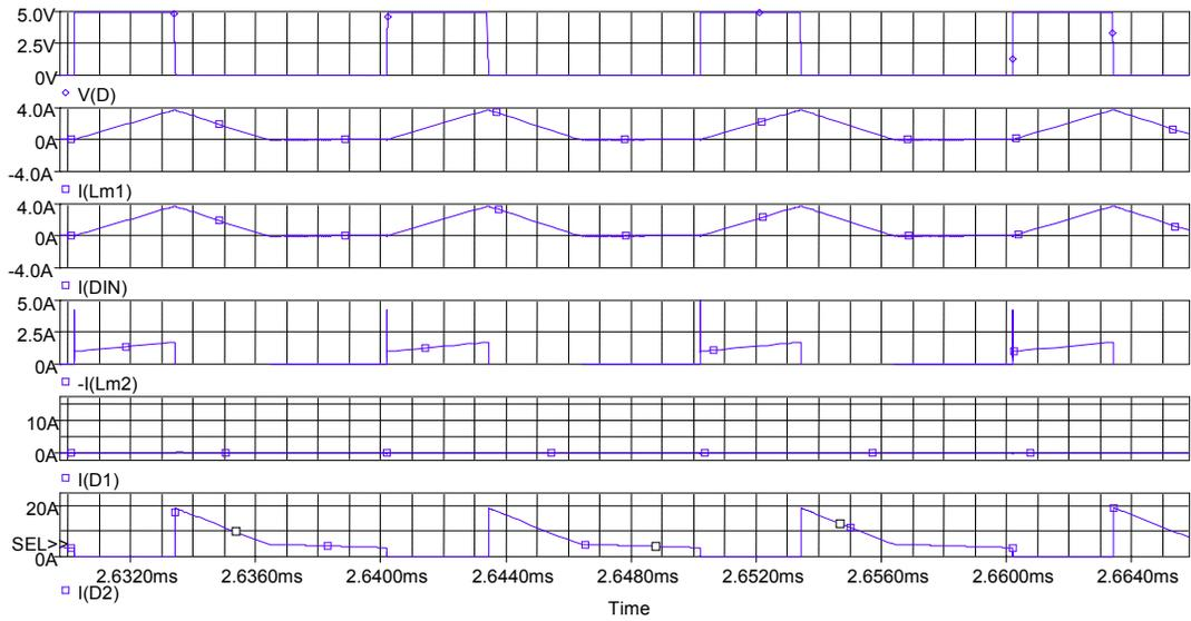
Figure 4-21 Simulation Waveforms during the Boost Mode
