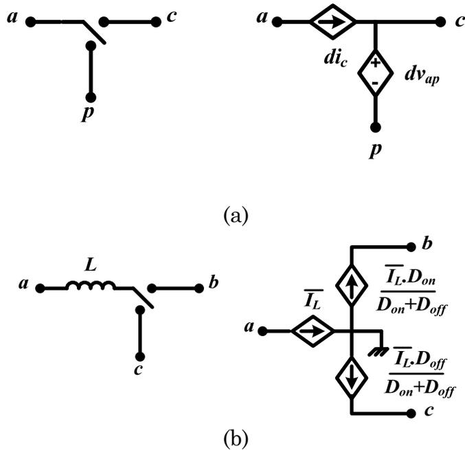
Figure 5-1 Switch Models (a) PWM Switch, (b) GSIM
