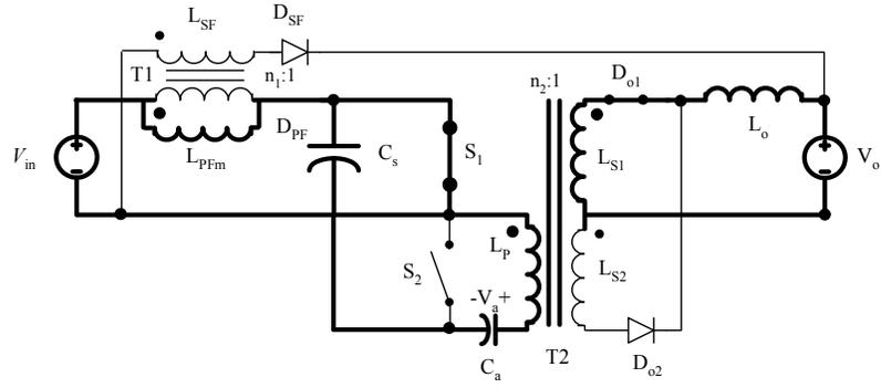
(a) Mode 1:  $t_0 < t < t_1$
