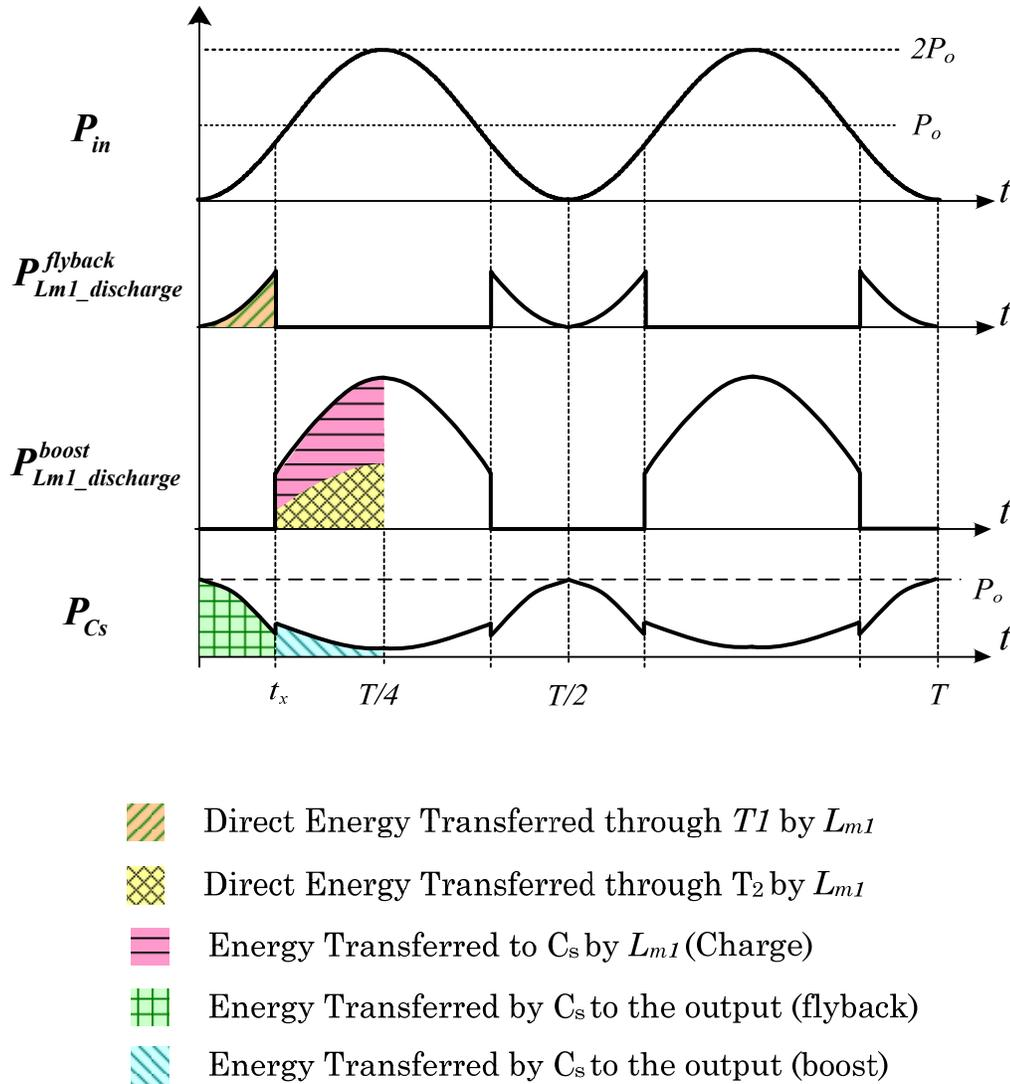
Figure 4-8 Power Flow Over a line cycle
