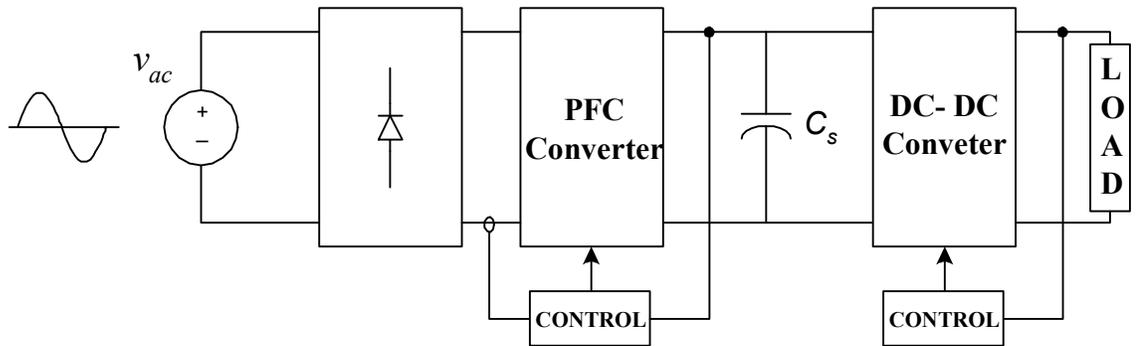
Figure 1-5 System Configuration of Two-stage PFC Power Supply
