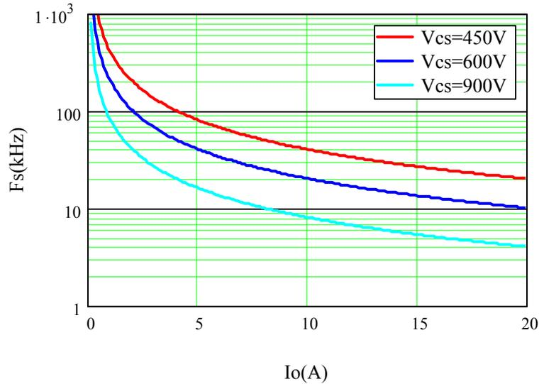
Figure 2-2 Switching Frequency vs. Load Current
