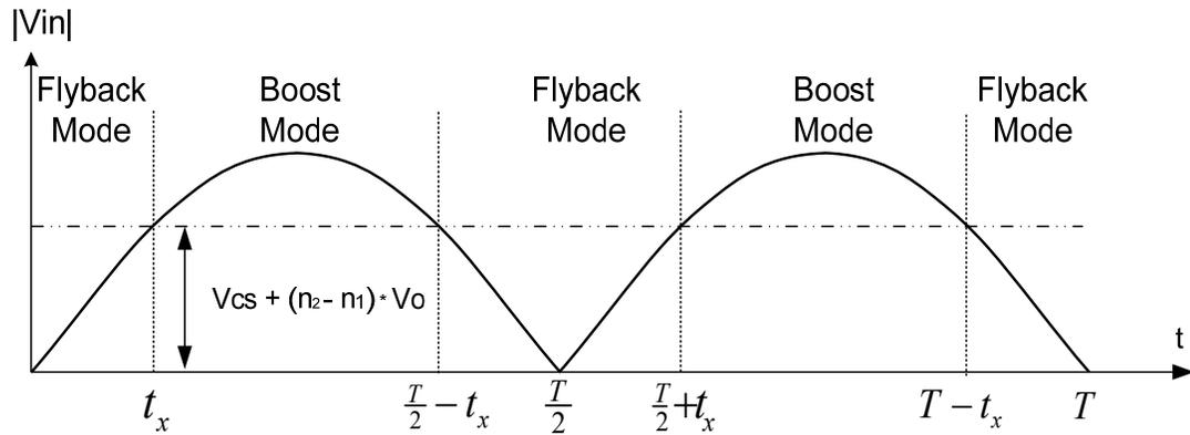
Figure 4-3 Modes of Operation during a Line Cycle
