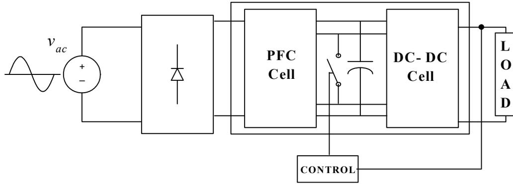
Figure 1-6 System Configuration of Single-stage PFC Power Supply
