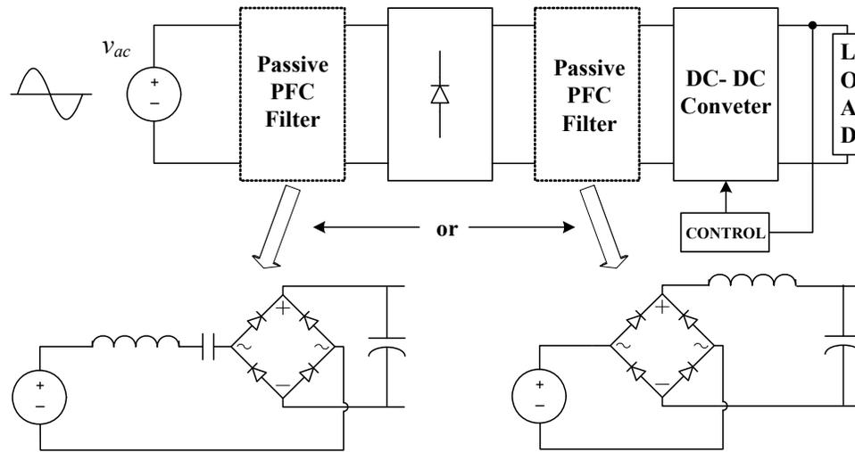
Figure 1-3 General Structures of the Passive PFC Approaches
