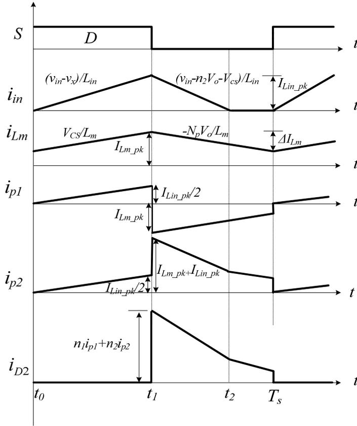
Figure 6-6 Key Waveforms during Mode 2 Operation
