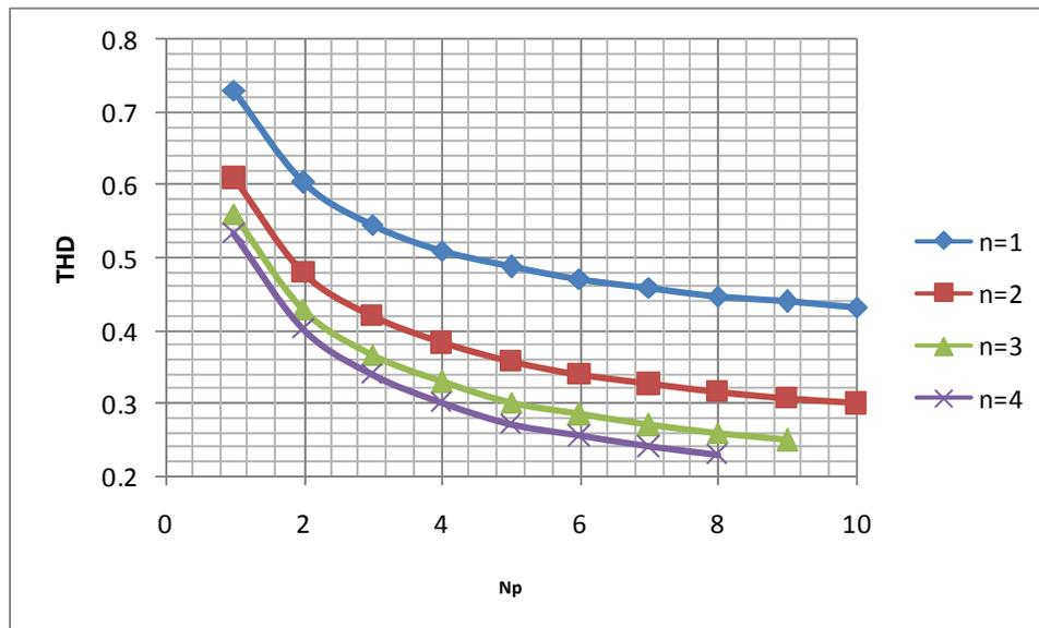
Figure 6-10 THD versus  $N_p$  for Different  $N$  Values
