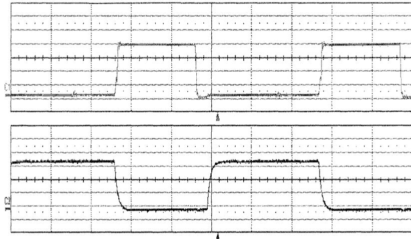
Fig. 2.20. ZVS waveforms of switch S_3
