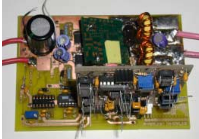
Fig. 3.16 The power stage of the proposed peak current mode controlled DC-DC converter
