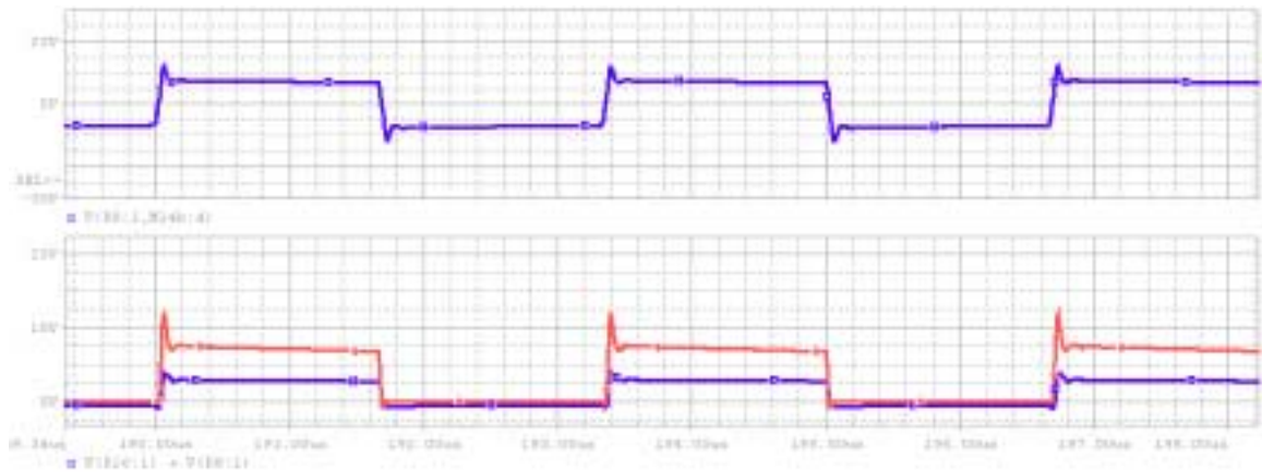
Fig. 5.37 (a) 36V converter input voltage
