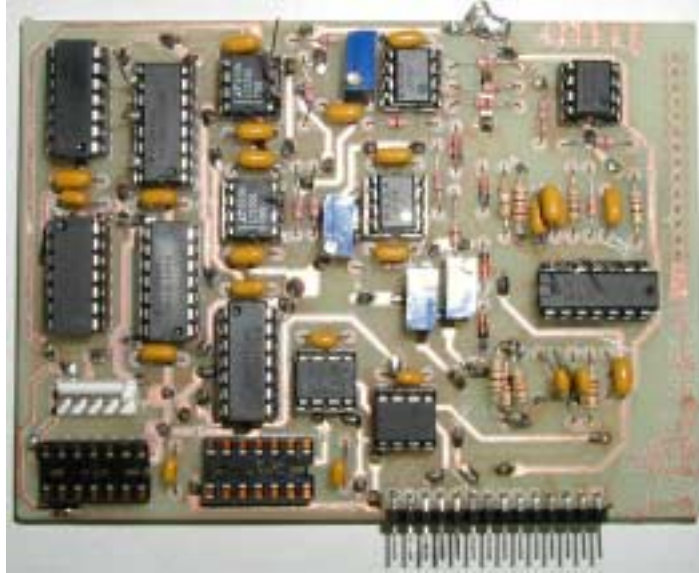
Fig. 3.18 The control board employing proposed peak current mode control scheme for symmetric half-bridge
