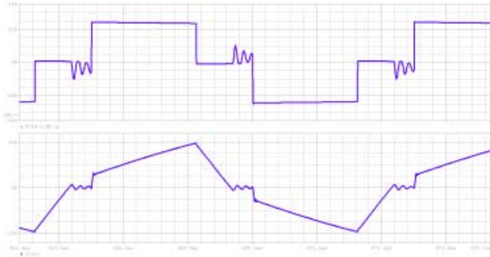
Fig. 5.17 (c) With active-clamp snubber ( C_s=3\mu\text{F} )
