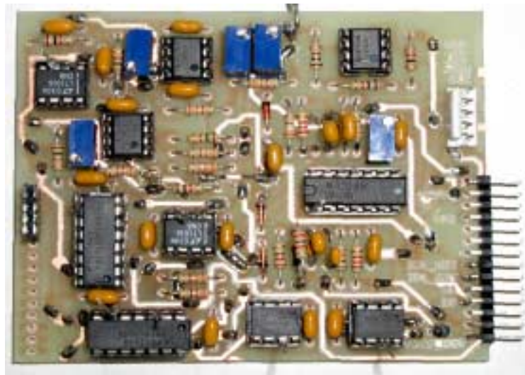
Fig. 3.17 The control board employing proposed peak current mode control scheme for DCS half-bridge topology
